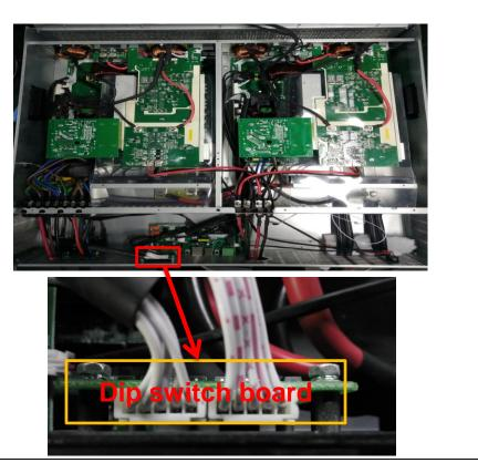
Please check the cables on the two control boards also.
