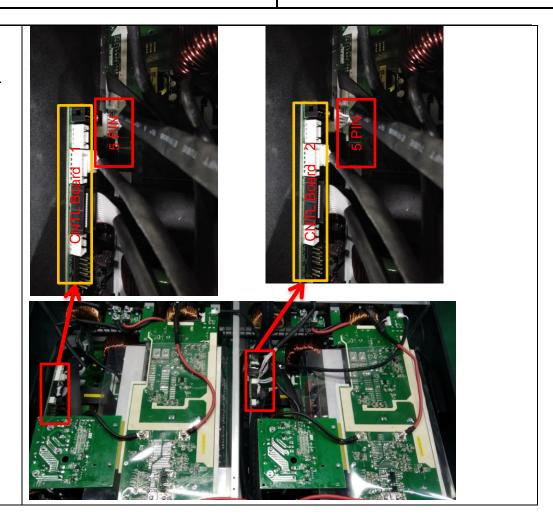
If the connection is OK, the possible issue is the dip switch board; you can change the board to solve it.
